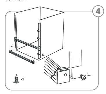
4) Align the bottom bar assembly with the bottom corners and floor panel of the habitat. Carefully guide the bottom panel and corners into the slot in the bottom bar assembly. Insert the sheet metal screws into both sides (a.) and (b.).
