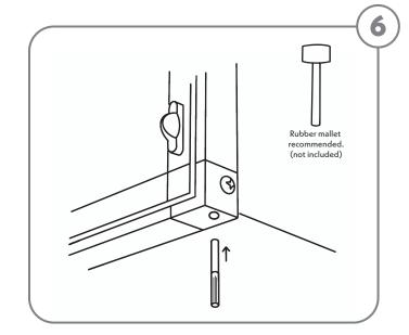
6) Push the Alignment Pin into the hole on the bottom front right-hand corner of the habitat until flush with frame rail.
