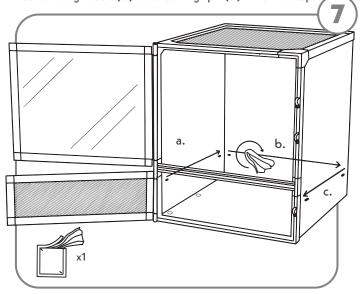
7) **Optional:** If installing Bioactive Retention Tray, prepare the habitat by wiping along the inside walls (a.) (b.) (c.) at the level of the rivet holes thoroughly with the included primer wipe.
