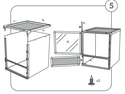
5) Align the top assembly frame with the top of habitat walls. Starting at one back corner, carefully press the slot in the frame onto the habitat top, making sure all sides are flush with the walls of the habitat. Insert the three sheet metal screws around the left, right, and back of the frame affixing the top to the walls (a.) (b.) (c.). After installing the top, insert and align doors (d.) and slide hinge pin (e.) in from the top.
