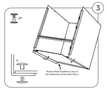
3) Pre-fold the bottom floor tabs on the main habitat panel inwards; bottom panel should be installed on top of folded side tabs as shown in diagram (a.). Begin inserting the top and bottom rivets around the  $\,$ perimeter until all nine holes on the bottom panel are affixed to the main habitat panel.
