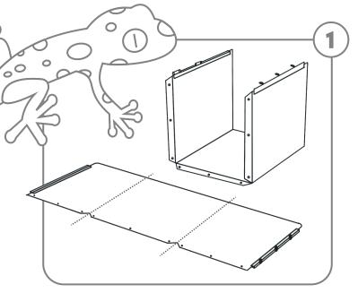
1) Lay the full flat main panel face down on a table, unfolded. Fold the panels forward (towards the decal) on the triangular indent lines. (Using the side of a table helps cleanly crease the folds)
