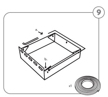
9) Remove backing from one side of the adhesive strip. Affix the strip around the back three sides of the tray (a.) starting at the top right side directly behind the cut-out dot (b.) and above the rivet holes.
