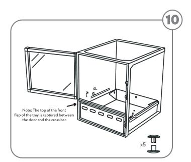
10) Open the bottom door of the habitat and insert the tray. Remove the outer backing of the adhesive strip (a.) and make sure that the adhesive strip creates a complete seal between the tray and the walls of the habitat. Next, attach the five rivets through the holes in the outer wall of the habitat and into the inside of the aligned holes on the tray, securing the inside corner folds of the tray.
