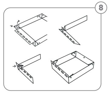
8) Bioactive Retention Tray Assembly: Fold the corners of the bottom tray inward on either side of the tray.
